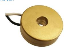
The Model 2GN is a highly accurate toroidal style current transformer designed to be used as testing and calibration standards as well as being used for energy monitoring out in the field. The core is made from the best magnetic alloy available to provide extremely low loss, good linearity and high sensitivity at low input currents. The 2GN is UL Listed under UL2808, Cat III. Sentran Corporation has the file number E361441.
