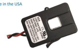
The Model LCDC is the transducer style of current transformer of the Model LC45. The LCDC is UL Recognized E318465. Due to the small size, the LCDC has a 100A maximum input current, making it ideal for monitoring cramped locations such as control panels.
